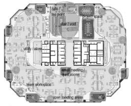
Figure 2: Zoning in a typical floor - Stockland Head Office, Sydney (Source: Bligh Voller Nield Architecture)
